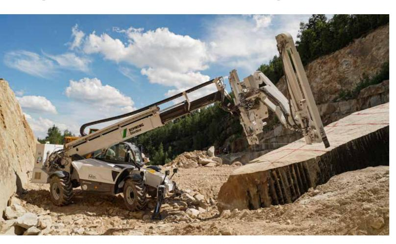
With its agility, cutting quality and compact design, the MDS revolutionises the processing of raw blocks in natural stone quarrying. The wire saw unit stands out with its considerable cutting capacity and compact transport dimensions without additional conversion effort. The machine is fully hydraulic; there are no electric actuators. To optimise the cutting capacity and cutting quality, particular attention was paid to the stability and the number of wire deflection pulleys.
