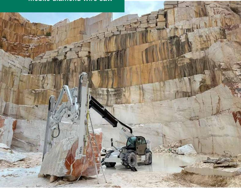
$\begin{array}{ll} \text{Cutting width} & < 5 \text{ m} \\ \text{Cutting depth} & < 3,4 \text{ m} \end{array}$
